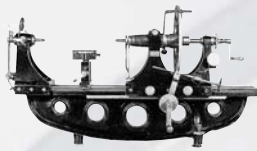
Length measuring machine from 1908. Reading on the vernier 1/10,000 mm
